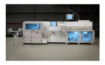
The Hauni Straw Maker allows you to produce visually appealing, high-quality, biodegradable straws. They have a smooth surface without overlapping paper, are food-safe and contain only minimal amounts of adhesive. Thanks to the market-proven, high-tech HSM process, you only need one type of paper to produce the straws, thereby saving material:
